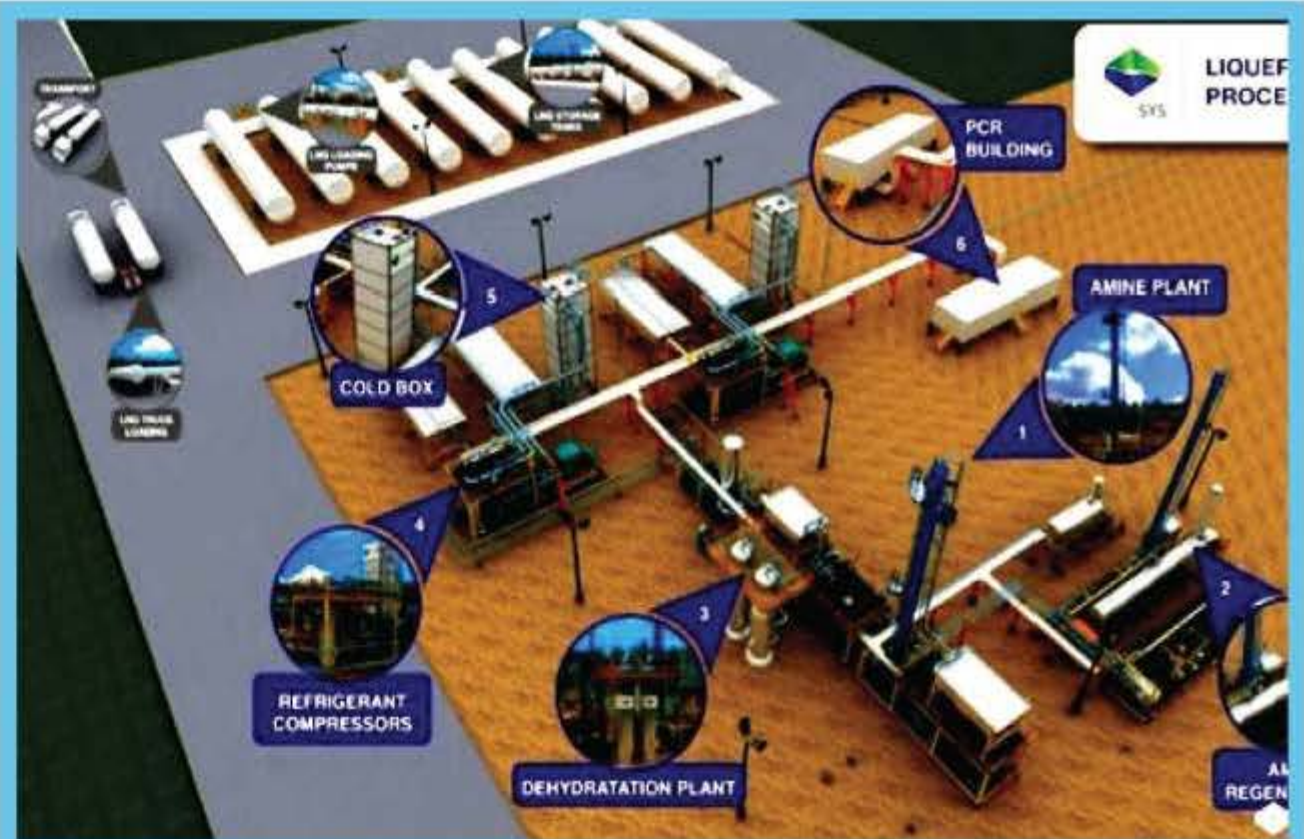
Train-1 Will Process up to 10MMSCFD
